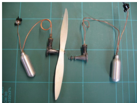
Pair of Brown Junior 0.005 motors. Telco fillers have been fitted to suit my charger nozzles. These two are from the batch of 500 produced with Nylatron pistons around 1970.
